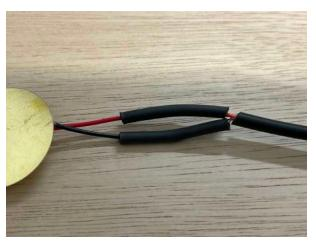
7 - AN ADULT then moves the longer/wider piece of heatshrink over the joins, and heats until it shrinks tightly - MAKE SURE there is a small gap between the heatshrink and the microphone element.
