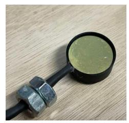
9 - Squeeze some warm glue where the cable joins the cap and quickly bring the first M10 nut down - carefully add some glue to fill any gaps
