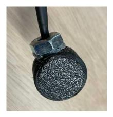
10 - Fill the gaps between the cable and the nut with glue, and add a bit more glue to stick the next M10 nut down on top of the first one. Fill in the gap between the cable and the second nut, then carefully fill in the gaps between the nuts. Try not to leave any gaps - this needs to be sturdy and waterproof.
