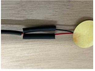
6 - AN ADULT will use the heatgun to shrink the heatshrink tightly around the wires. ( Make sure the longer, wider length of heat shrink is not too close so it doesn't shrink too at this point.)
