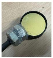
11 - Place a line of glue around the edge of the cap, making sure there are no gaps between the brass and the edge of the cap. THIS BIT IS REALLY IMPORTANT! - make sure there are no gaps. This is making it waterproof
